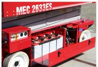
Dedicated lower control box centralizes components for easy access. Interchangeable with other MEC models.
