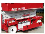
Dedicated lower control box centralizes components for easy access. Interchangeable with other MEC models.
