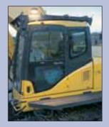
Step light with timer Provides light for about one minute to allow the operator to get off the machine safely.
