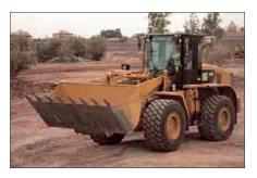
Constant Net Horsepower. On many competitive machines, gross horsepower is constant, meaning that net engine power available for actual work will vary based on demands made from parasitic sources, such as air conditioning or cooling fans.
