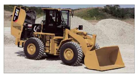
**Engine Compartment Access.**A single mechanical lift cylinder with manual back-up opens the hood. The tilting hood provides excellent
