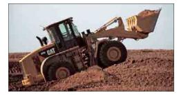
**Ride Control**. The optional Ride Control System improves ride, performance and load retention when traveling over rough terrain. Operators gain confidence moving at higher speeds in load and carry operations decreasing cycle times and increasing productivity.
